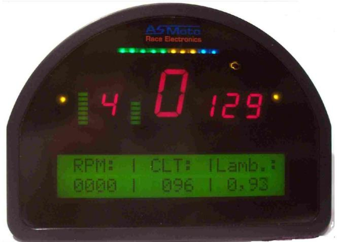
The second generation DashBoard LED instrument cluster was expanded with a multitude of new features. Thanks to the LED technology the display has a higher level of contrast so the most important information among all conditions can be read even without direct glance. Brightness of each segment can be separately programmed or switched off.
